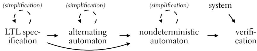
Fig. 1.1: The verification procedure for LTL as a series of translations
